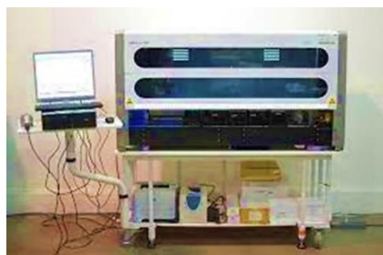
Figure 1 Cobas X 480 for quantitative detection of CMV virus
