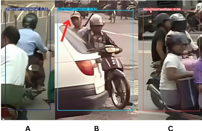
FIGURE 6. Sample failure cases of the MCVD model. Annotations A and C illustrate misclassifications in highly crowded scenes involving closely spaced motorcycles, while B shows confusion between a cap and a helmet for distant rider instances.
