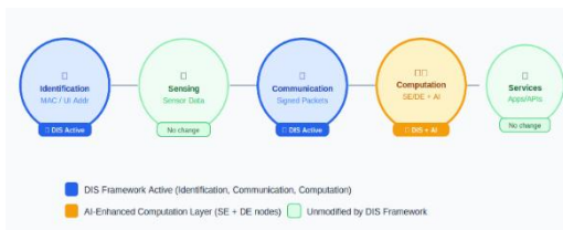
FIGURE 5: AI-DIS Interaction with IoT Architectural Elements. The six standard elements and where AI-DIS engages each one: MAC/UI addressing at Identification; signed-packet transport at Communication; HMAC and TinyML inference at Computation; authenticated stream delivery at Services.
