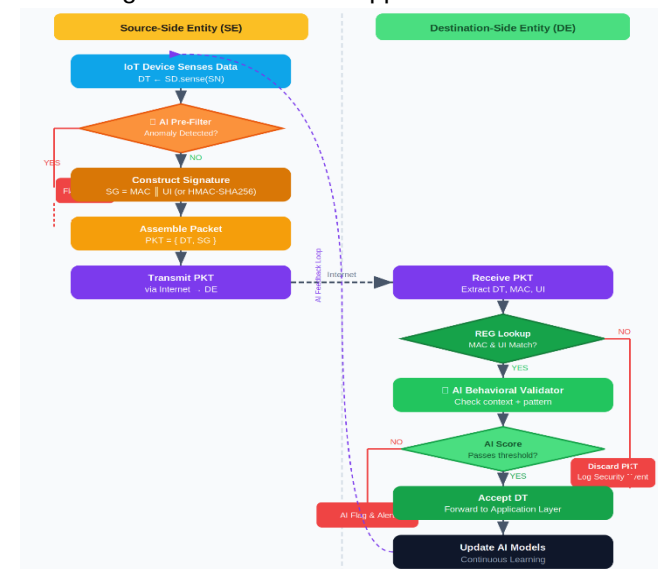
FIGURE 4: AI-DIS Operational Workflow. At the SE (left), each reading passes the TinyML pre-filter before the HMAC-SHA256 signature is formed and the packet is dispatched. At the DE (right), the replay guard runs first, followed by signature verification and the AI behavioural validator, before the reading reaches the application. The dashed loop shows the periodic FedAvg model-update path.
