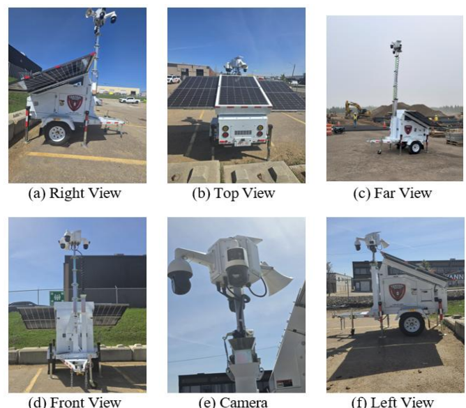
Figure 4: CCTV Tower Close-up View. (a) Right View (b) Top View (c) Far View (d) Front View (e) Camera (f) Left View
