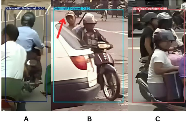
FIGURE 6. Sample failure cases of the MCVD model. Annotations A and C illustrate misclassifications in highly crowded scenes involving closely spaced motorcycles, while B shows confusion between a cap and a helmet for distant rider instances.
